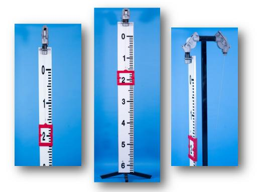
The GSI 2530 Liquid Level Indicator (Target Board) provides reliable and an inexpensive method for indication of the tank product LEVEL. A weighted target traveling a ruled board on the side of the tank is connected by cable to a float inside the tank, as the float moves up or down with product movement, the target correspondingly travels up or down the ruled target board on the outside of the tank.
